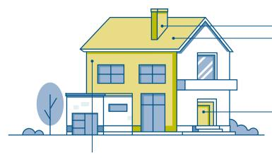
**CHIMNEY:** Cover your chimney outlet and stovepipe with a nonflammable screen of ½ inch mesh.
